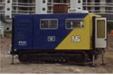
To supplement the existing geotechnical study, Morris-Shea performed an extensive program of cone testing to allow a better evaluation of the soft soils, and variability of the shelly sand bearing layer.
