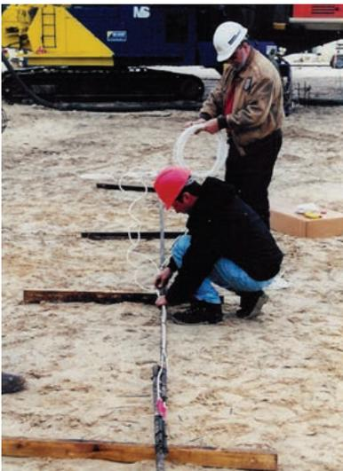
Two 1000-ton static jacks were used, together with a 1600-ton load frame to perform static testing. A MEGADEC data storage system was used to monitor load cell, strain gauge, and LVDT measurements, backed up with dial gauges and jack pressure measurements.
