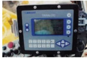
optimize pile length and provide quality assurance during pile construction. Key parameters such as drill depth, turntable torque, and drill rate are measured and displayed in-cab, allowing required pile tip depth to be verified on a pile by pile basis.
