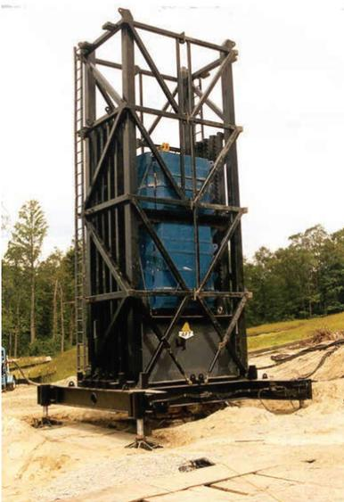
Installation criteria derived from load testing required minimum socket lengths in the limestone, with structure specific borings and drill rates being used to verify acceptability on a pile by pile basis.
