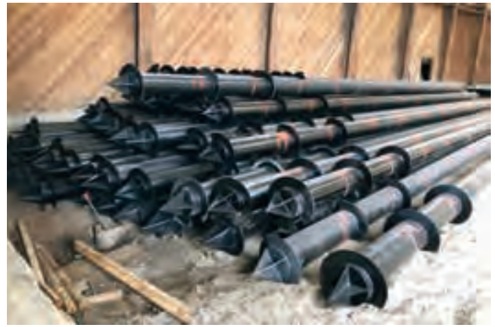
PC-CIDH steel casings with fabricated pile points
